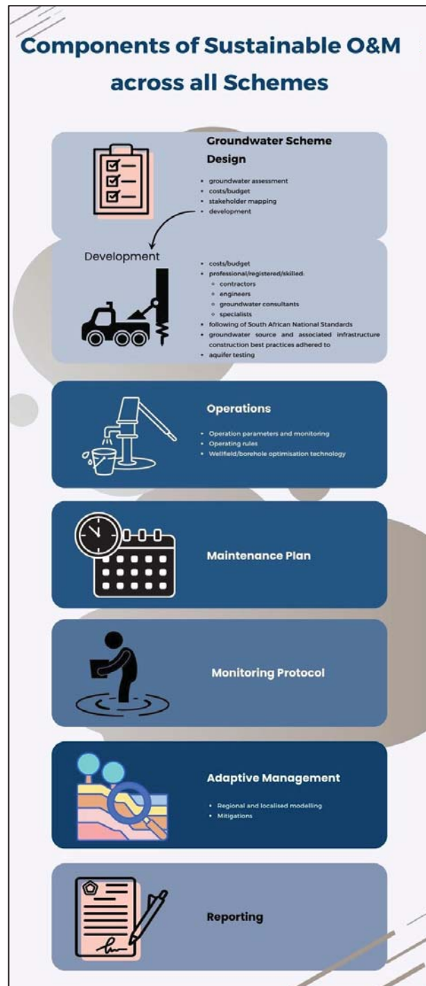
Figure 4-1 Overview of the key aspects of a sustainable O&M applicable across various groundwater schemes.
